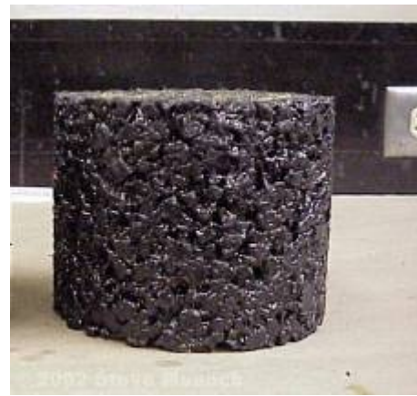
Stone Matrix Asphalt Lab Sample
