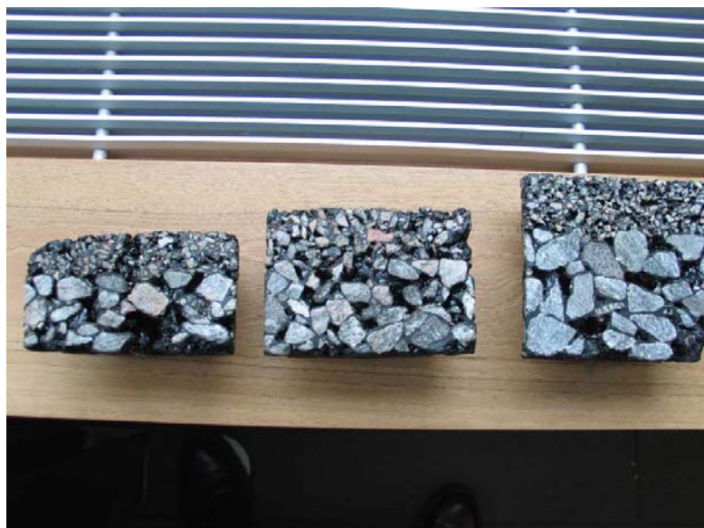
Examples of two-layer porous asphalt
